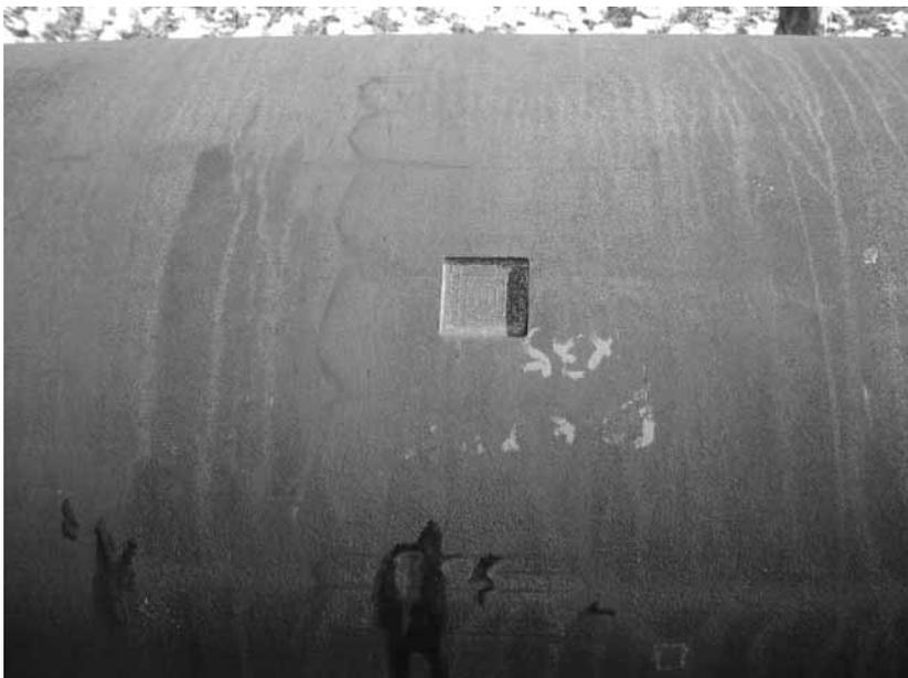
Fig. 6.10 3t×3t×0.2t defect[6]
