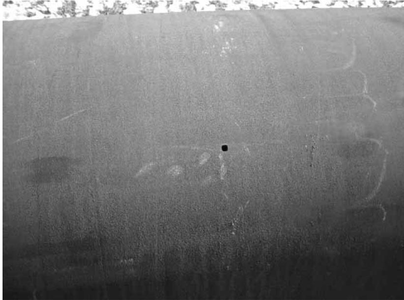
Fig. 6.11  $0.5t \times 0.5t \times \text{hole}$  defect[6]
