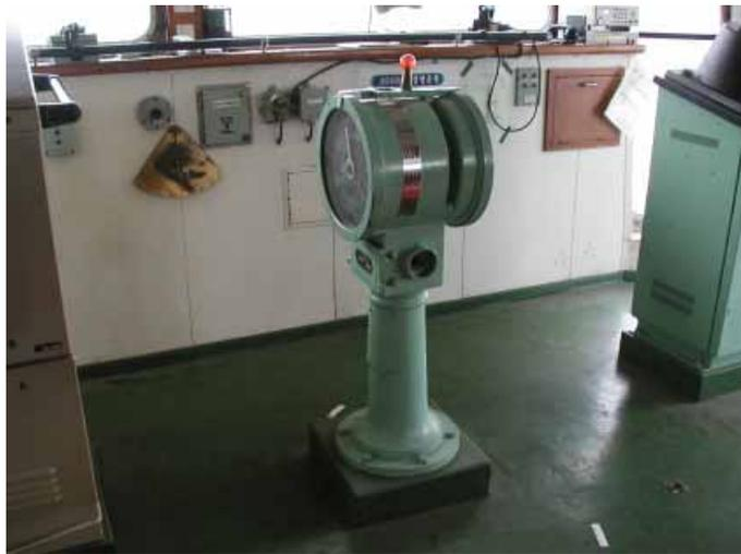
[Fig. 5-3] Inside view of bridge showing stand-alone engine telegraph
