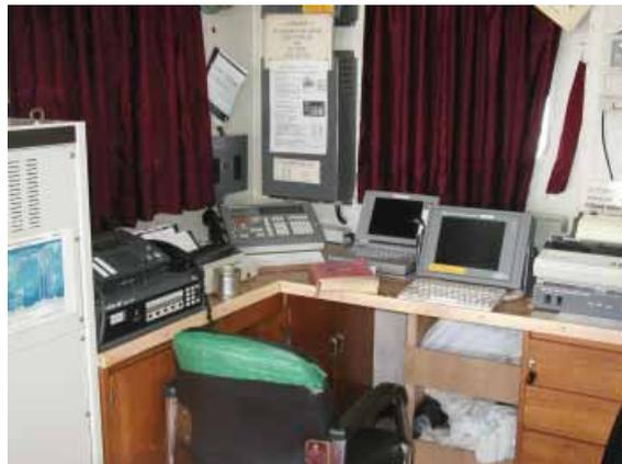
[Fig. 5-5] Various GMDSS equipment without ergonomic concept
