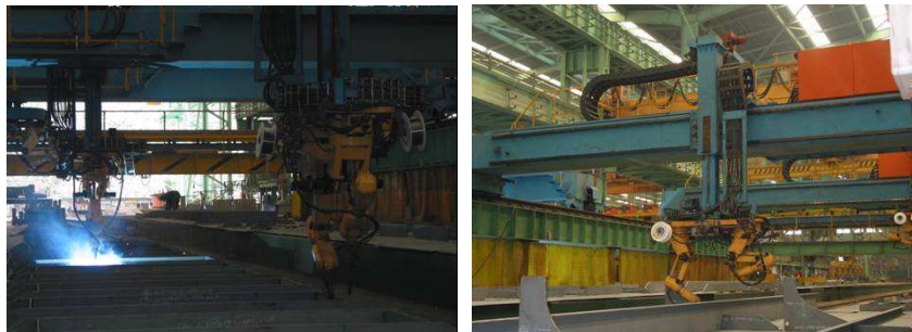
Fig. 2.3 Robot Welding Shop and gantry-robot
