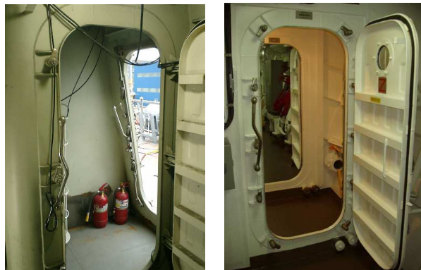
Fig. 4.23 Type I and III air lock for naval ship
