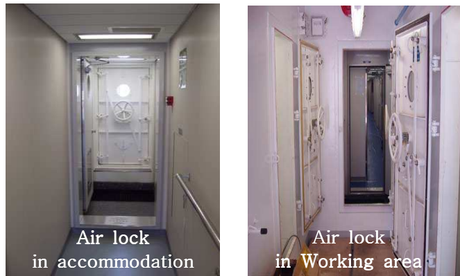
Fig. 4.15 Air lock in working area and accommodation
