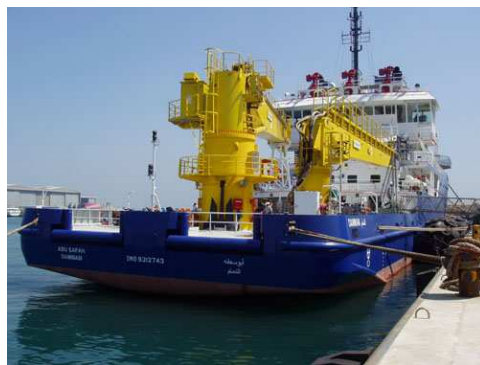
Fig. 4.13 Well services maintenance support vessel
