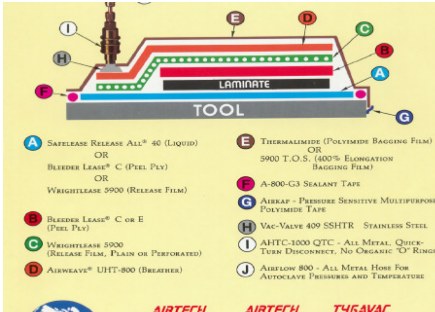
Fig. 10 Lay-up of vacuum bagging materials.
