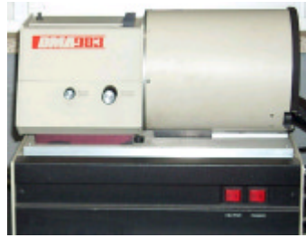
Fig. 24 DMA983 (Dynamic mechanical analysis).
