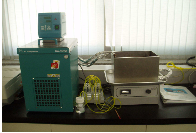
Fig. 3.2 Aerobic respirometer for the biodegradability test (AER 204)
