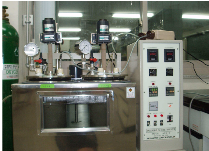
Fig. 3.3 Anaerobic/aerobic bioreactor for the organics in the sediment
