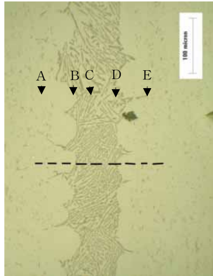
Photo. 5 Optical microstructure of cross section brazed at 863K for 180s, 300s, 420s
