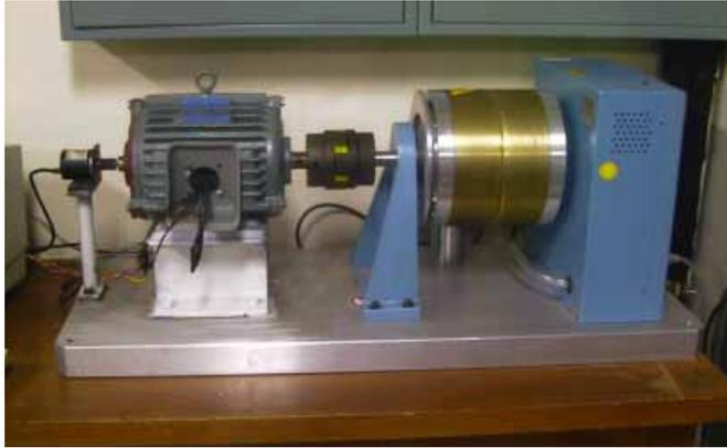
Fig. 6.6 Induction motor and Dynamometer of the experimental equipment
