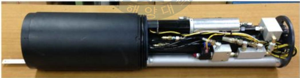
Fig. 3.8 Buoyancy engine
