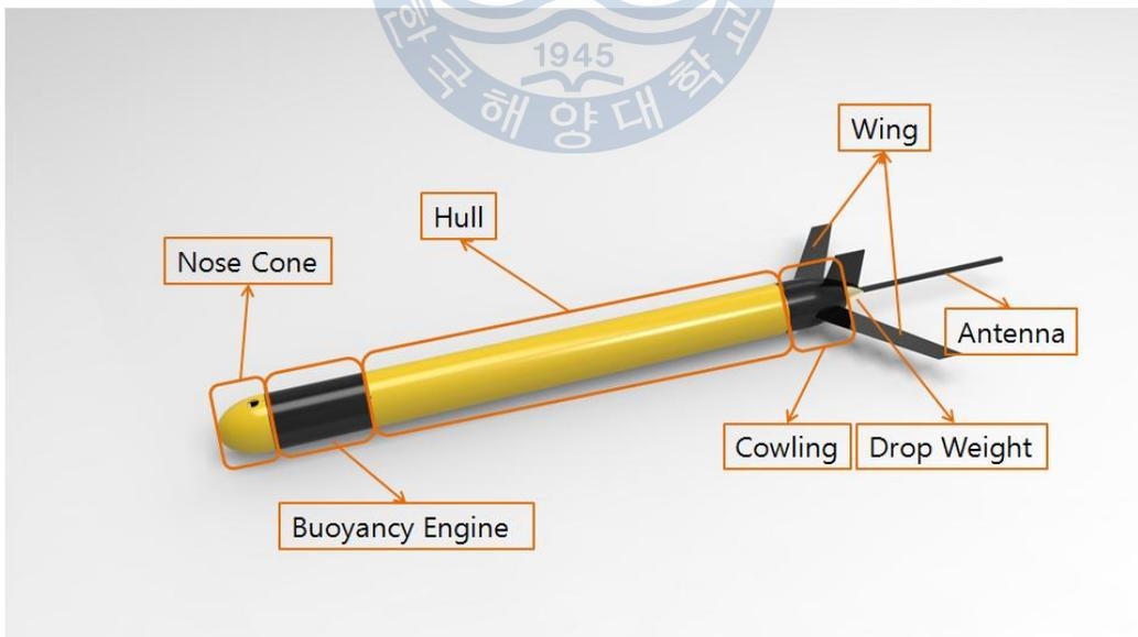
Fig. 2.1 External shape of underwater glider
