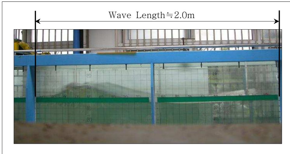
Photo 4.1 Scene of Estimating Wave Length in Breaking Wave
