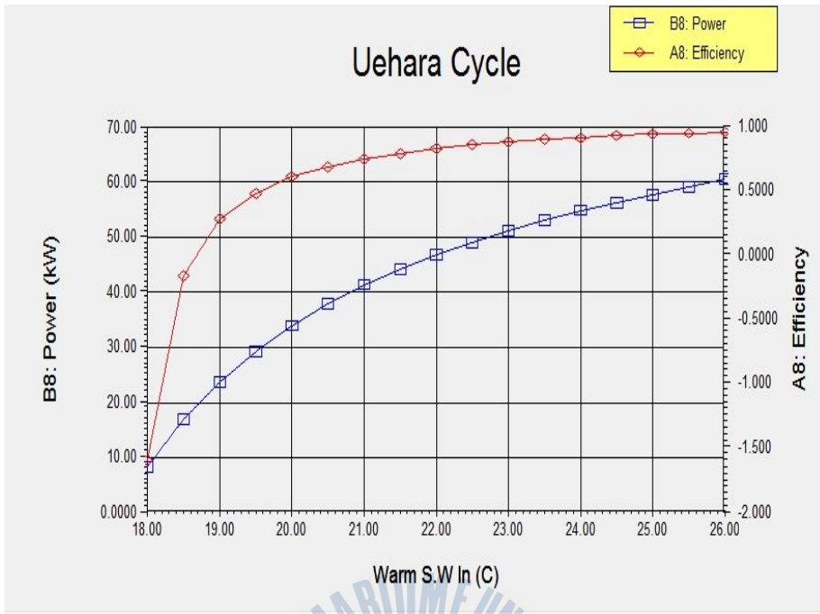
Fig. 4-36 : Power and efficiency of the cycle according to surface seawater temperature(Uehara cycle)
