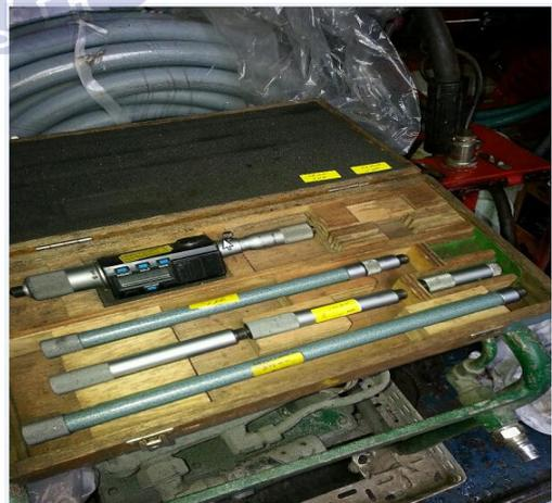
Fig.4.8 Micrometer for measurement
