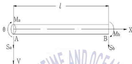
Fig. 3.2 Coordinate system of beam-element and forces of end-section
