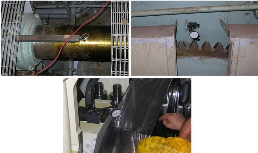
Fig. 3.11 Measurement of bearing load by jack up method
