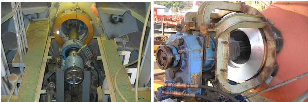
Fig.4.6 Stern tube boring machine
