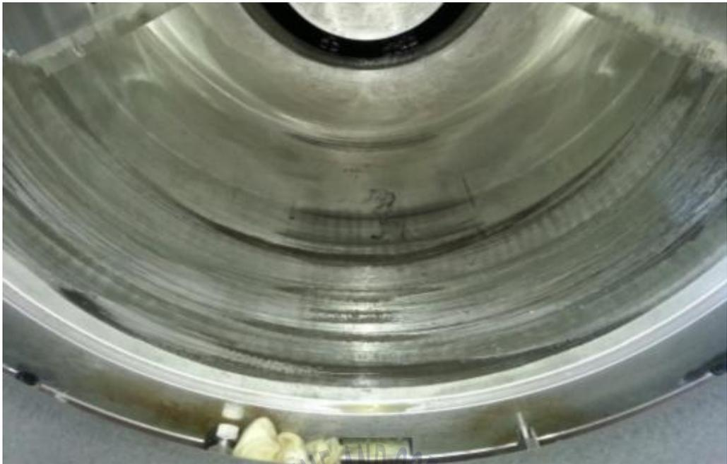
Fig. 4.19 The condition of stern tube forward bearing
