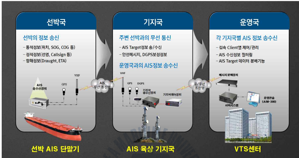
Fig. 2.1 AIS Operation System
