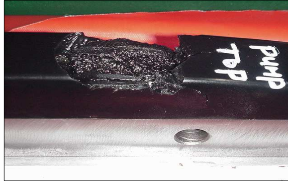
Fig. 2.8 Damaged guide bar by excessive vibration of roller chain
