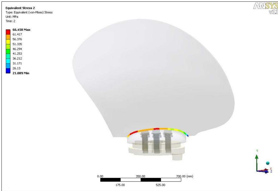
Fig. 3.6 Equivalent stress shape of the blade back at root in ahead condition
