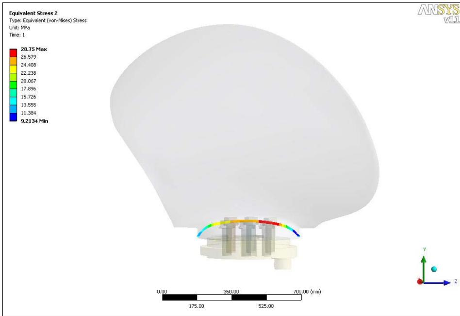
Fig. 3.11 Equivalent stress shape of the blade face at root in astern condition
