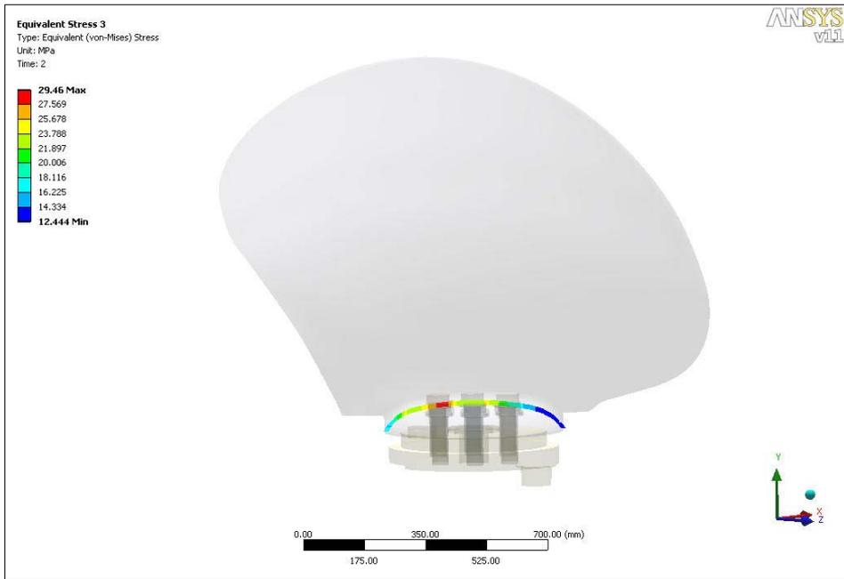
Fig. 3.4 Equivalent stress shape of the blade face at root in ahead condition
