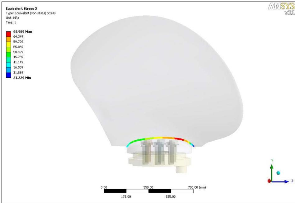
Fig. 3.13 Equivalent stress shape of the blade back at root in astern condition
