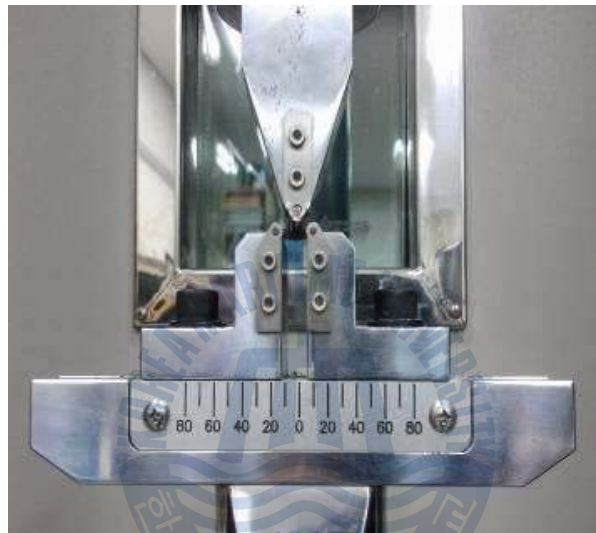
(c) Short beam test
