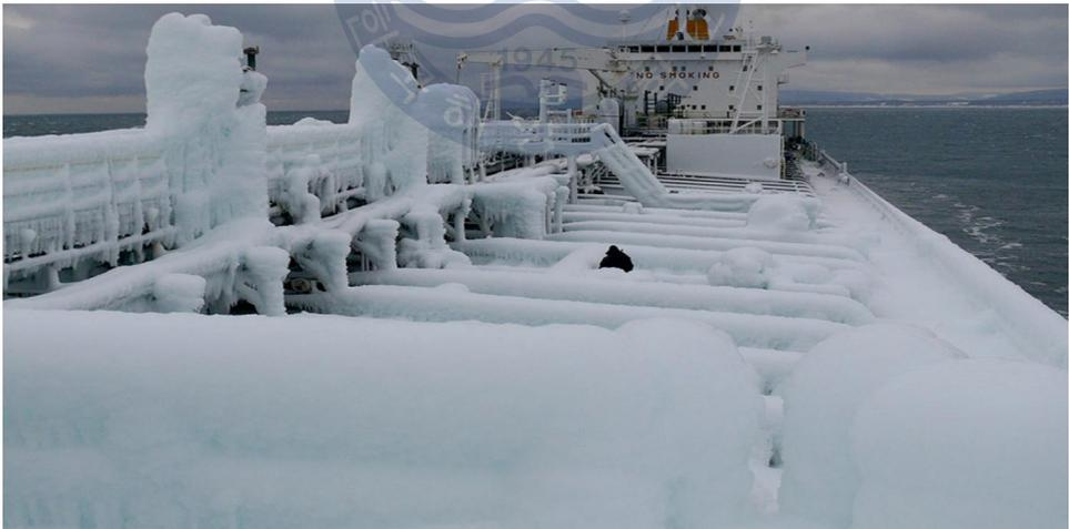
**Figure 2.9** Icing on deck(Source: www.groupocean.com)
