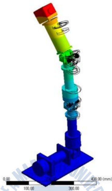
Fig 5.9 FEM displacement result of the manipulator – 3
