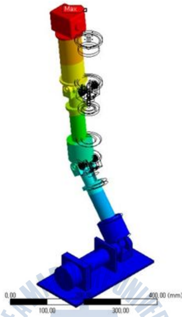
Fig 5.5 FEM displacement result of the manipulator – 1
