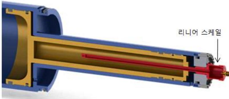
Fig. 2.12 Section view of buoyancy controller
