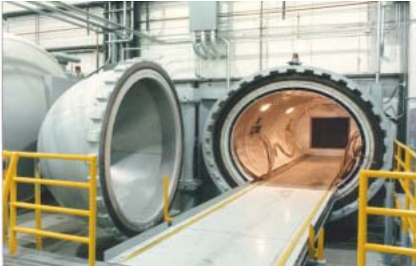
Fig. 22 The real shape of the used autoclave for laminate and sandwich panel process.
