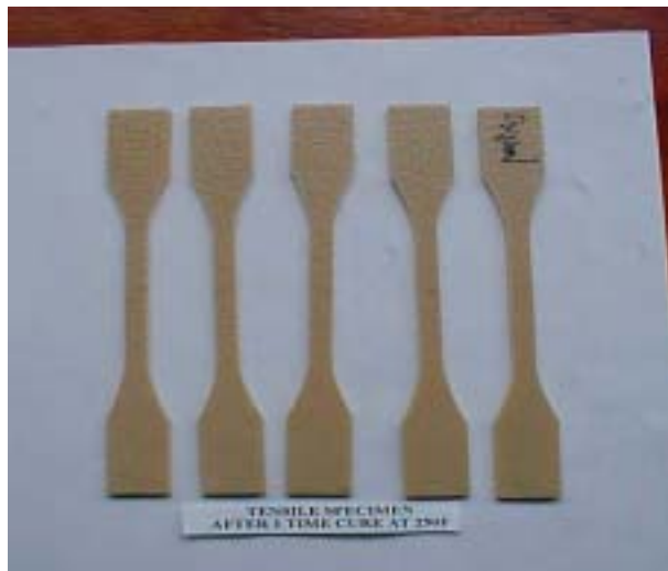
(a) Tensile specimen
