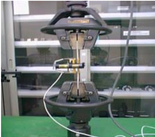
Fig. 25 The real shape of the used tensile test machine.
