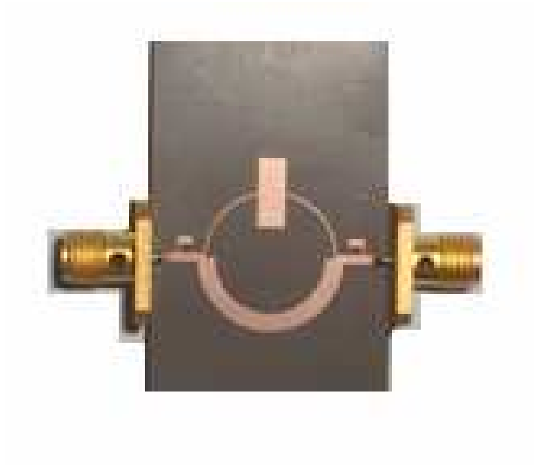
Fig. 3.12 The photograph of the proposed UWB filter.
