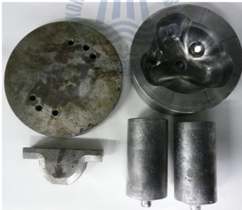
Fig. 35 Picture of experimental die sets
