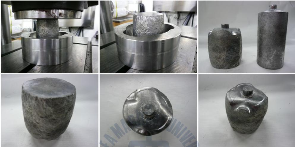
Fig. 36 Deformed shape after upsetting
