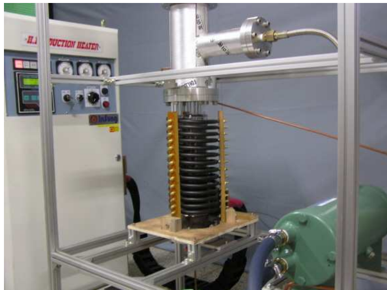
Figure 3. 2 H.F Induction Heater (Insung Co.)
