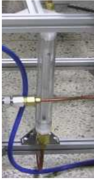
Figure 3. 9 Condensate flowmeter (OMEGA Co.)
