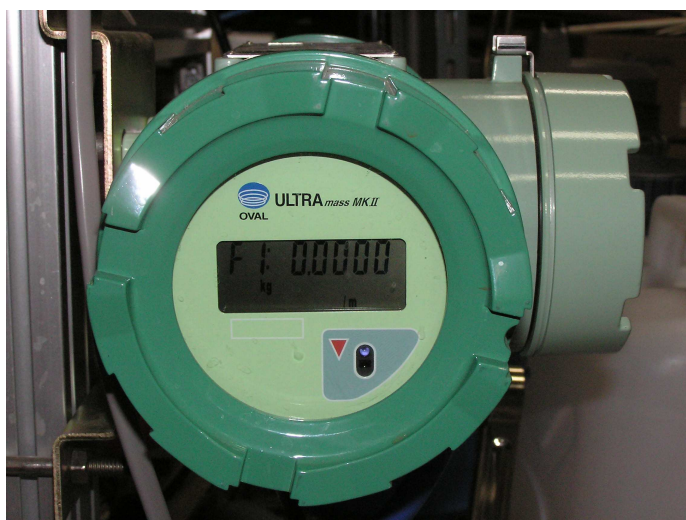
Figure 3. 8 Coriolis-type mass flow meter (OVAL Co.)
