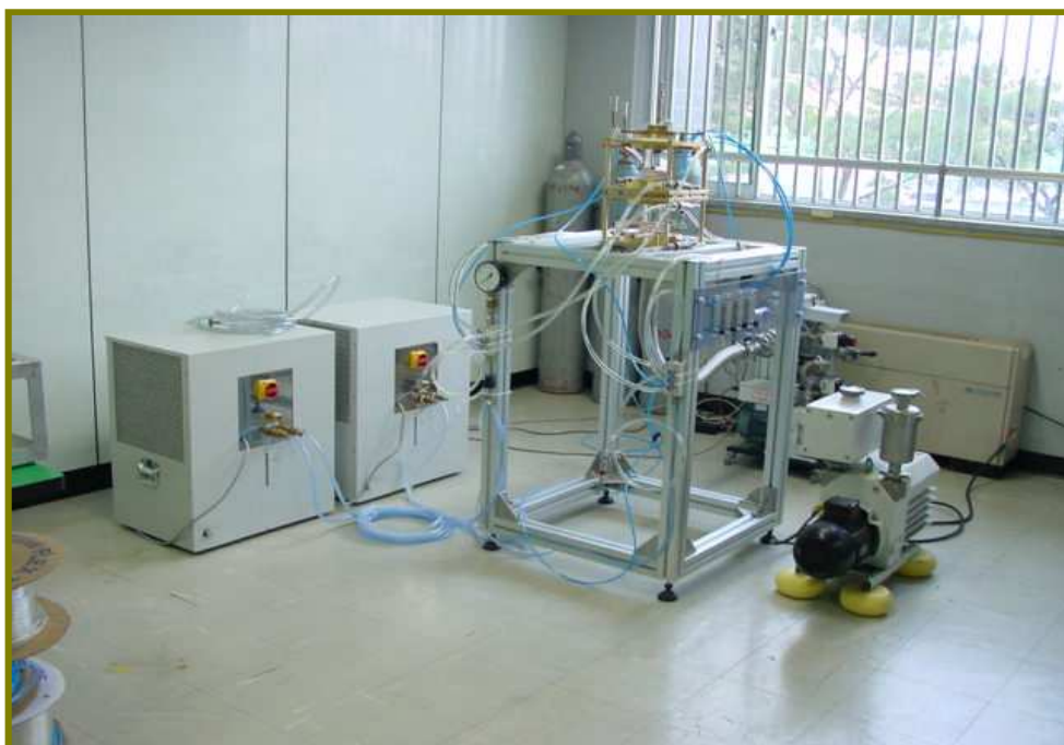
Fig. 2.4 A equipment which generates RF plazma inducted by 13.56MHz high frequency
