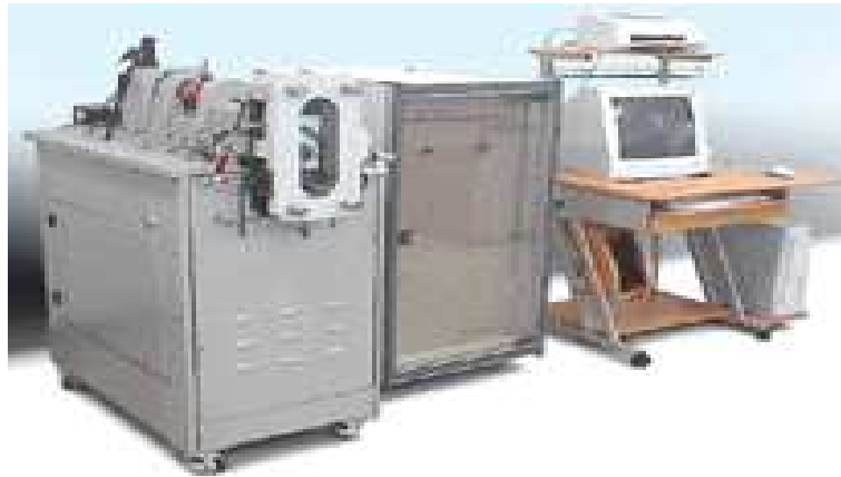
Fig. 4.1 Model of high speed rolling contact wear test machine
