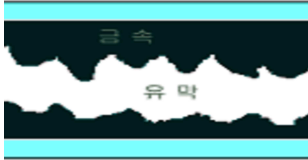
Fig. 3.1 Schematic of full-film lubrication
