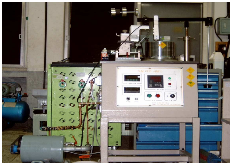
Fig. 4.24 Schematic diagram and photo of wear test machine
