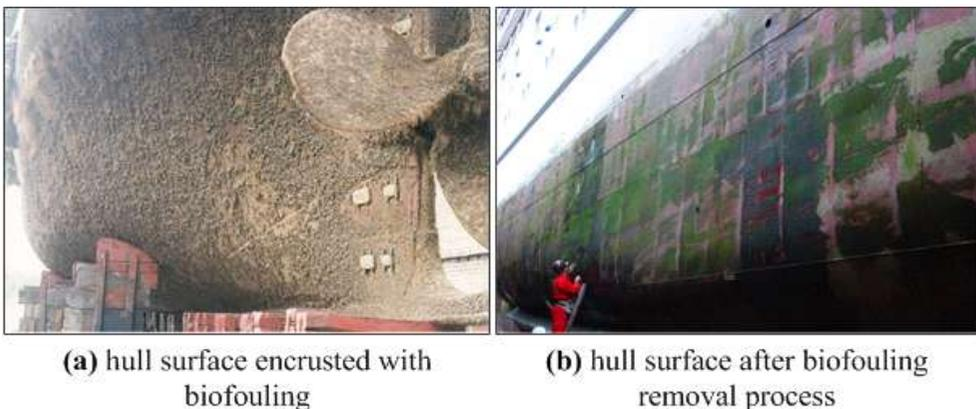
Fig 2.1 Hull surface conditions
