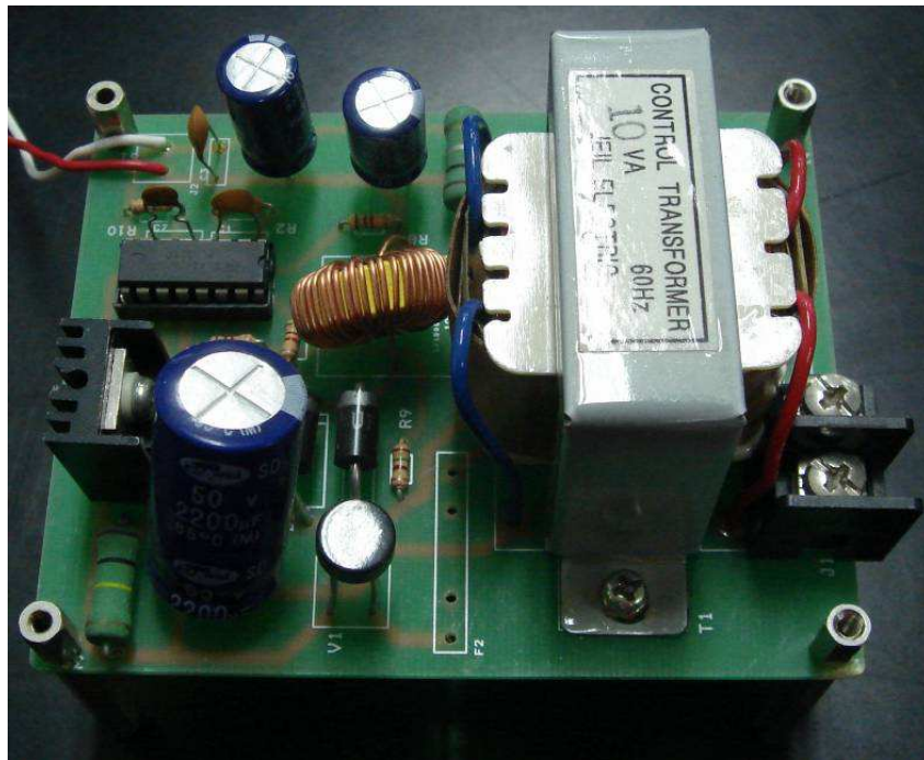
(a) Buck Converter System with Transformer
