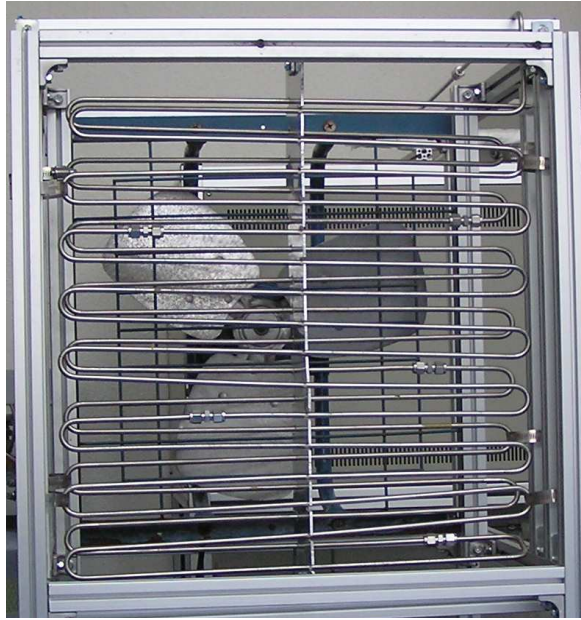
Fig. 3.3 Photograph of cooler
