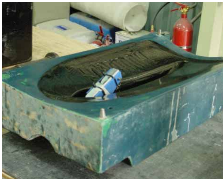
(c) Installed pad and jig for combining cylinder
