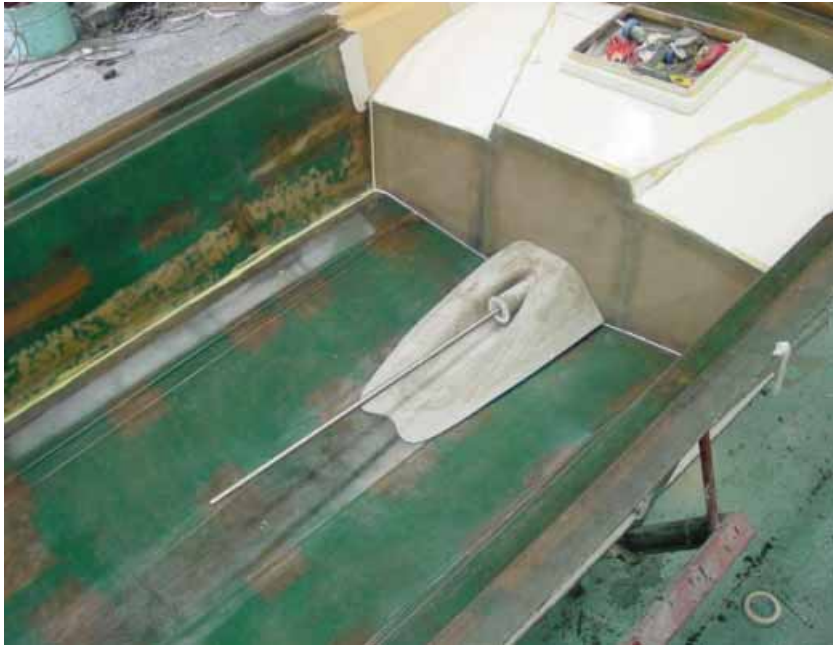
(c) Assembly between tunnel part and small boat body
