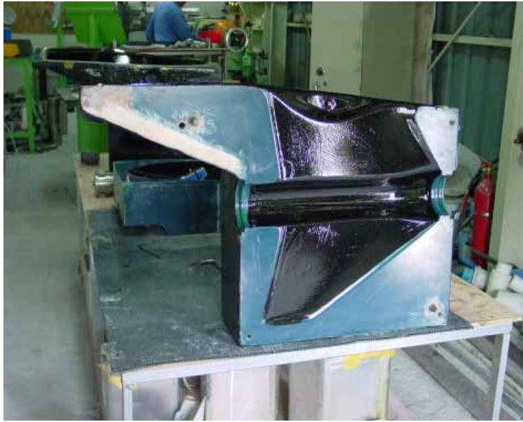
(a) Manufacturing mold
