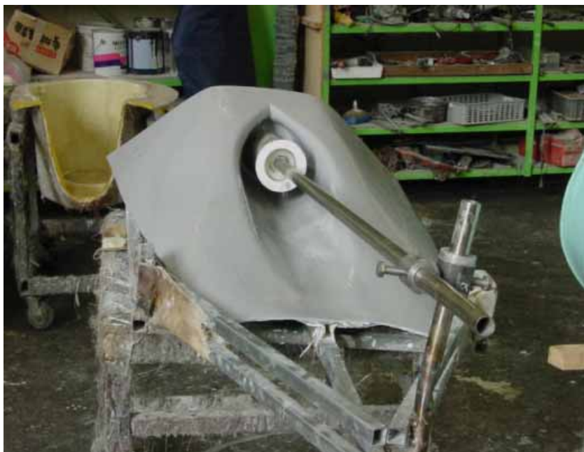
(b) Fabrication of tunnel part
