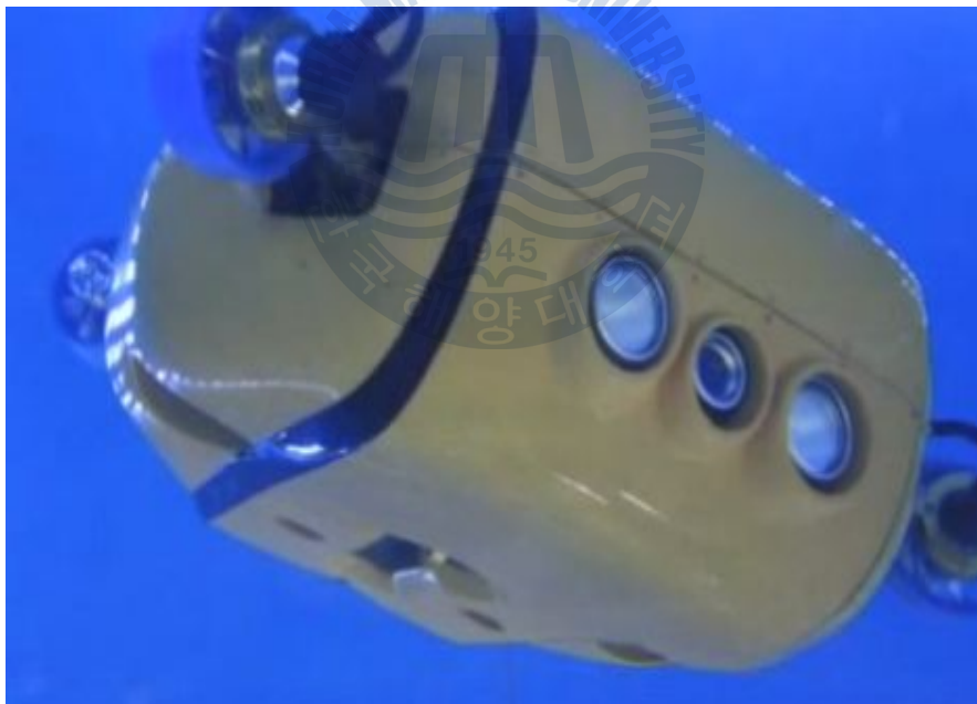
Fig 5.9 The actual 30 ° roll control test photo(in water pool)
