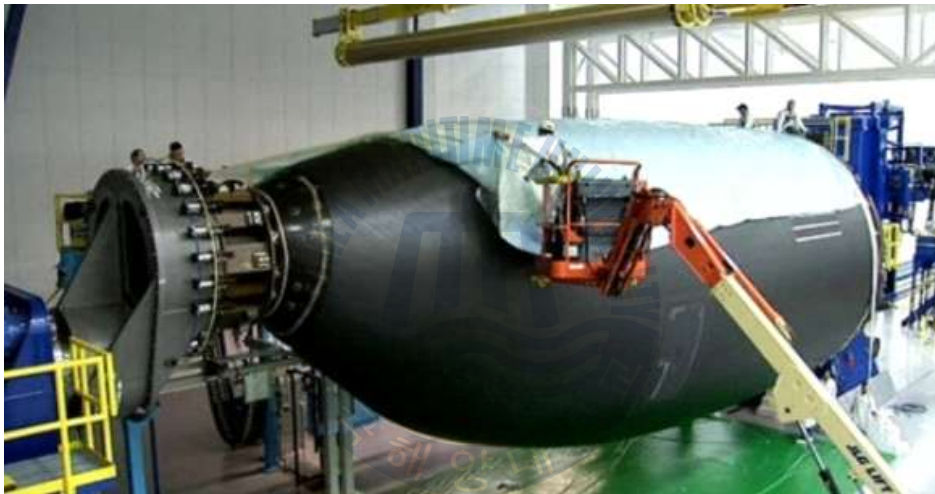
Fig. 3 Boeing 787 air plane parts with CFRP
