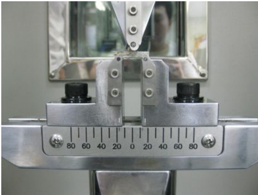
Fig. 3.5 Images of method for short-beam test
