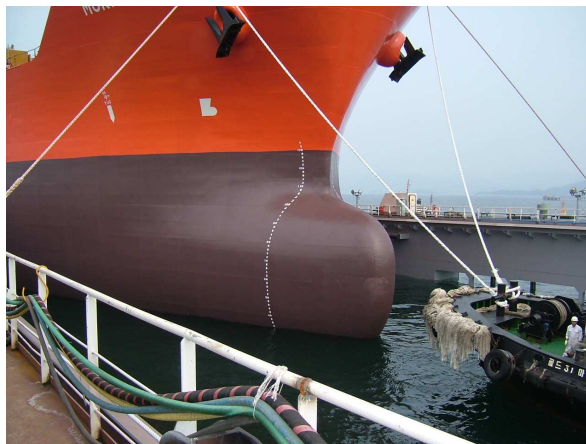
Fig. 6.8 Launching to Floating Dock
