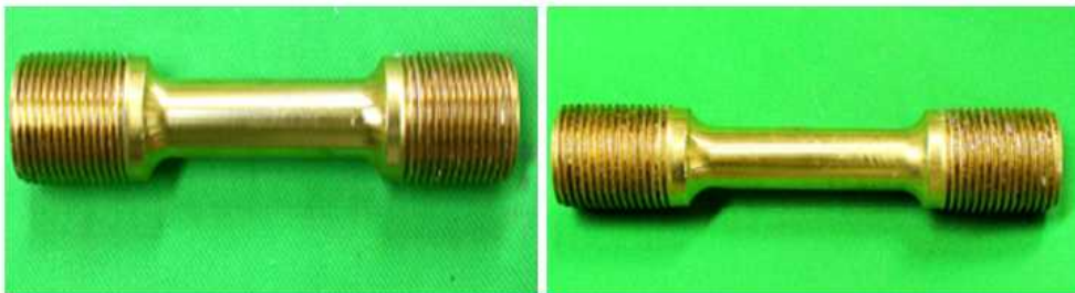
<Fig. 4.28> Neutral salt spray test result of Ti/TiN bolt (45min)
