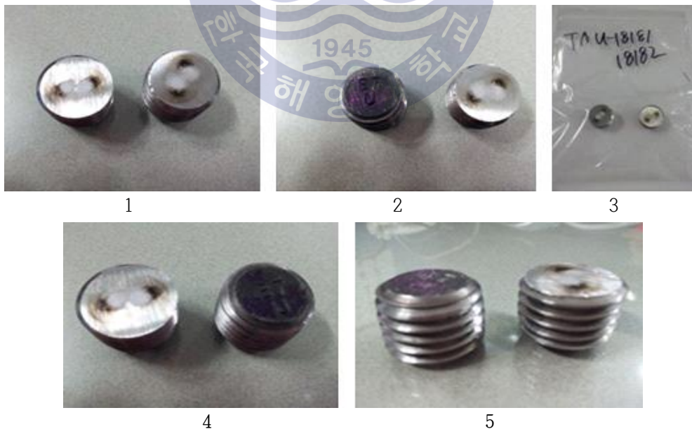
<Fig. 4.8> After testing B7 bolt A and B
