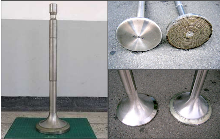
Fig. 3.4 A photo of Exhaust valve made by PTA process
