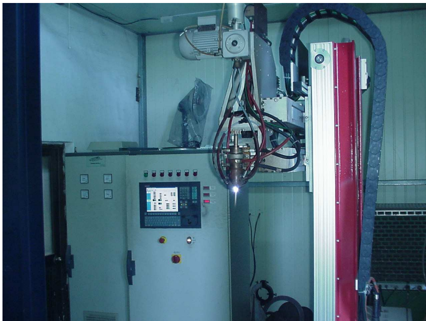
Fig. 3.3 PTA equipment and control panel of PTA
