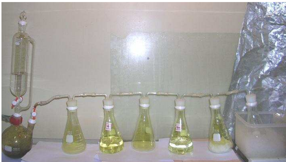
Figure 3.4. Experimental equipment for generating Cl 2 and KClO
