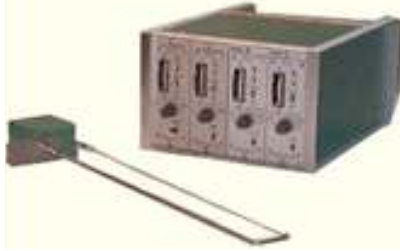
Fig.3.4. Capacity Type Wave Height Meter
