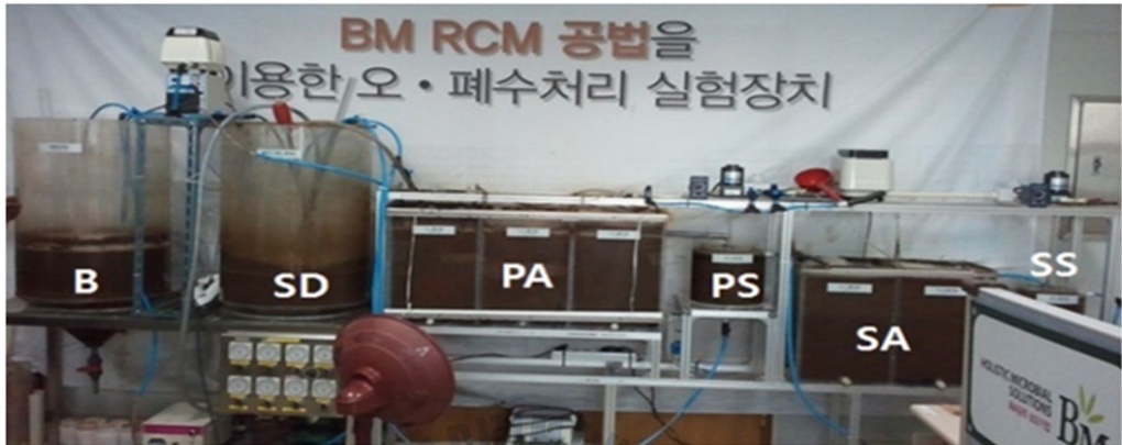
Fig. 7 Actual view of the pilot scale tannery wastewater treatment system
