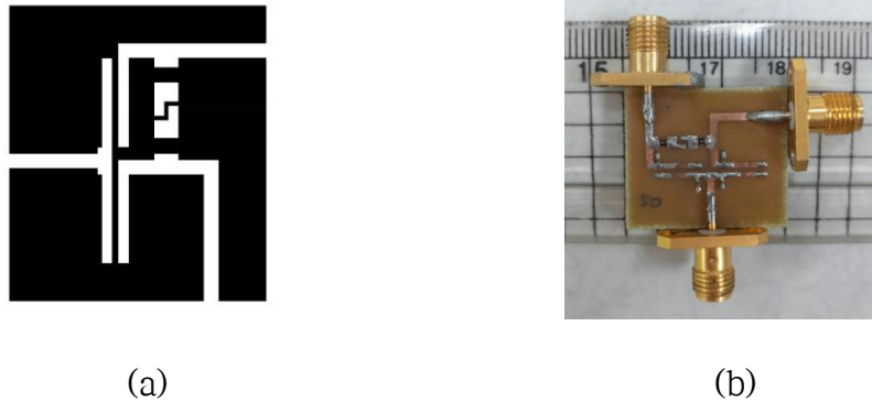
Fig.3.4 layout of two-stage fabrication circuit drawn through AutoCAD (a) and its photograph (b)
