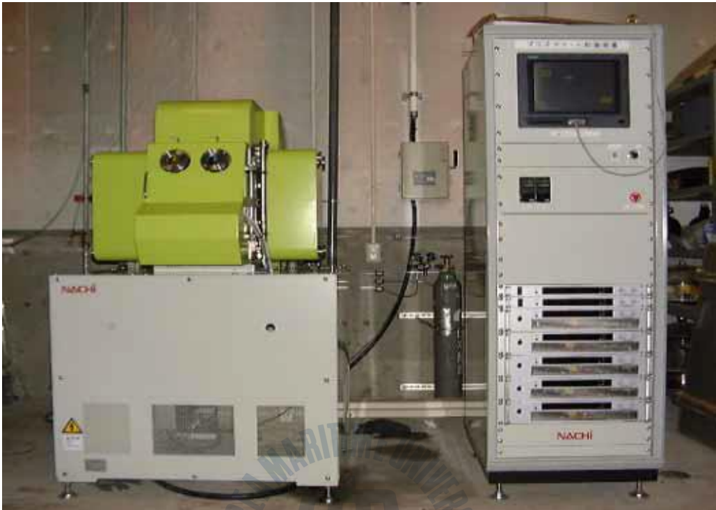
Fig. 3.1.1 The inclination opposite target type DC magnetron sputtering equipment
