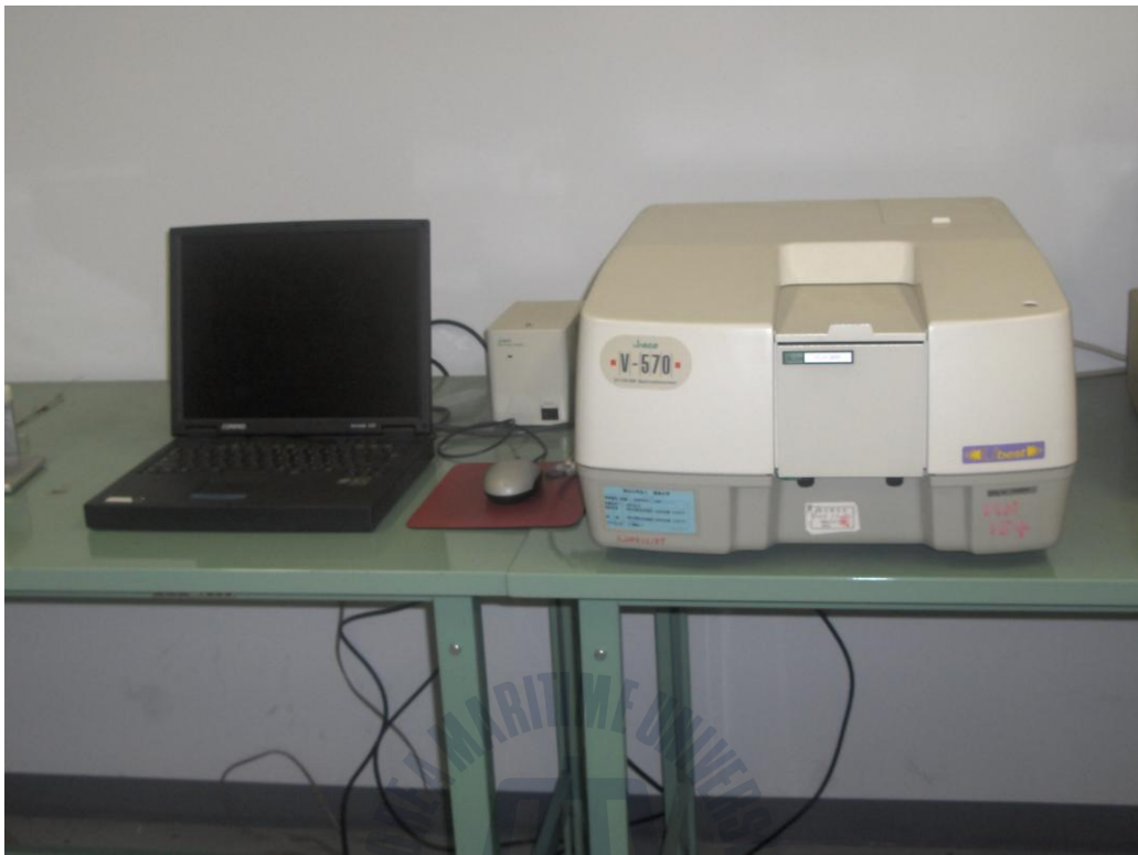
Fig. 3.2.2 The figure of UV-VIS-NIR spectrometer (V-570, Jasco)
