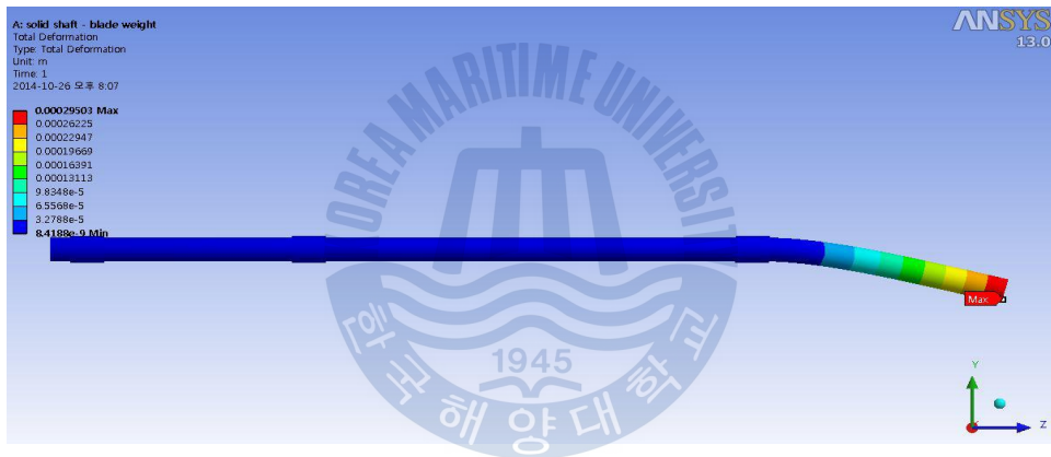
Fig. 3.4.7 Total deformation of shaft
