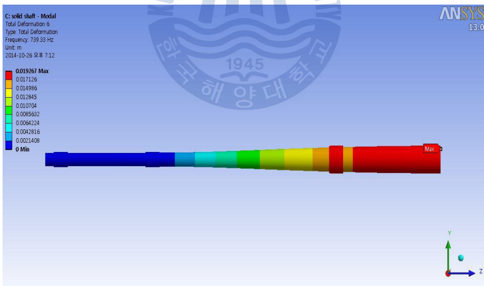
Fig. 3.4.17 The natural frequency of shaft (Mode 6)
