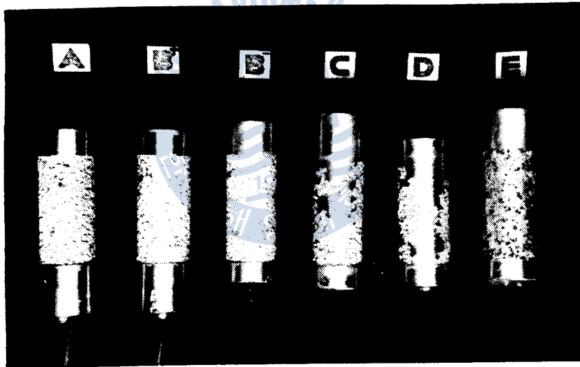
Fig.5 Corrosion Pattern of Anode Specimens
