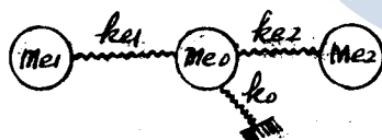
Fig. 2 The simplified equivalent system of the marine Diesel engine shafting
