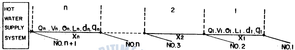
Fig. 4 Basic piping system
