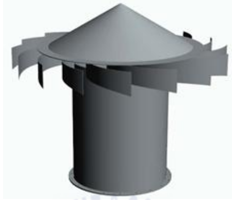
Fig. 3.4 Spray shielder & vane
