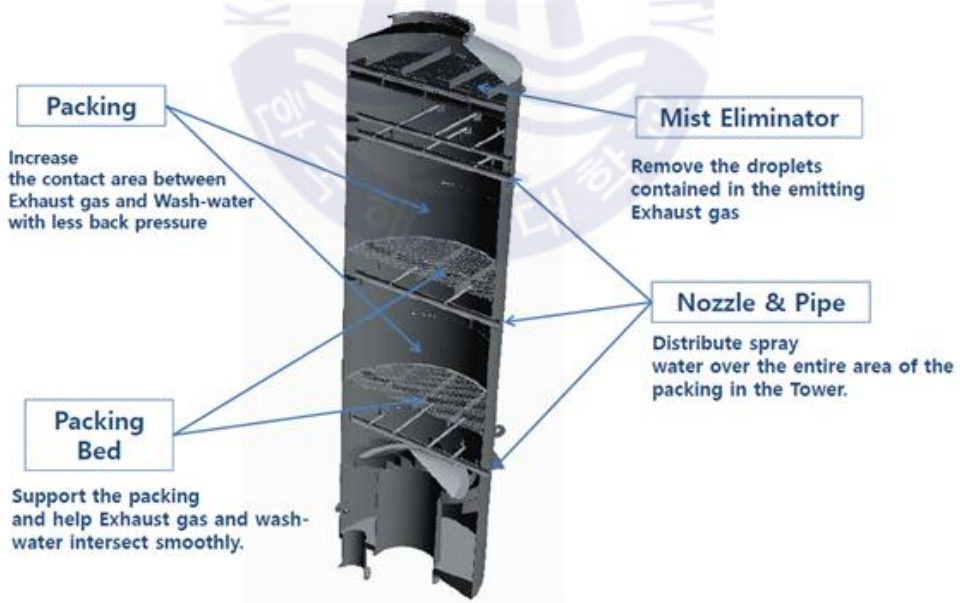
Fig. 3.3 Internal structure of SO x scrubber
