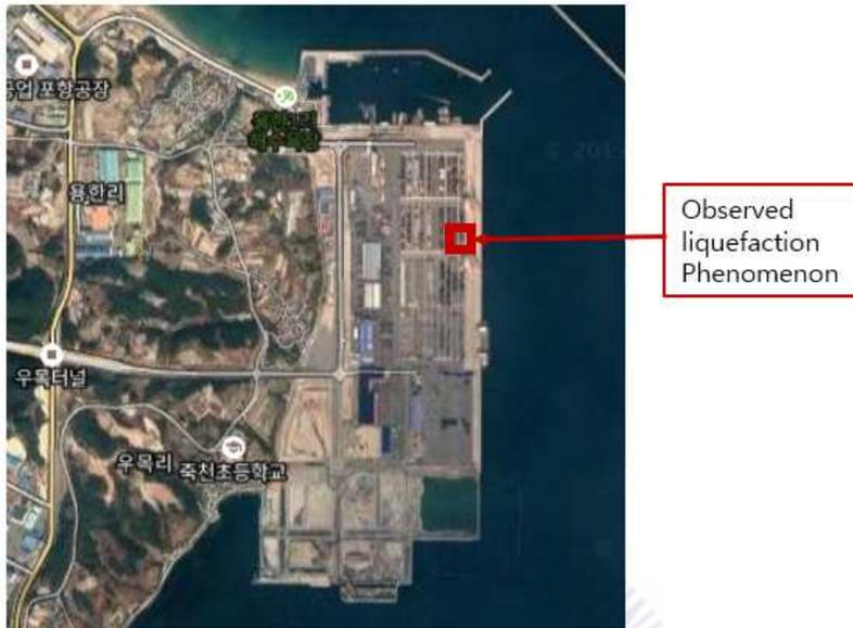
Fig. 4.1 Liquefaction location at Youngilman port during Pohang earthquake
