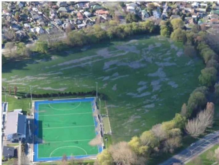
Fig. 1.2 Soil liquefaction occurred due to earthquake at Christchurch Porritt park in 2011 (Pender, M. et al., 2012)
