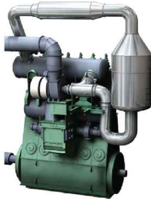
Fig. 2.3 Installation example of G/E SCR
