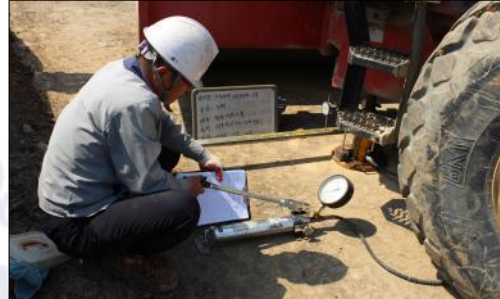
6. Plate load test
