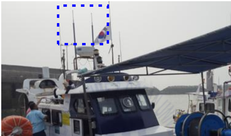
Fig. 10 Installation Location of the WAVE Antenna
