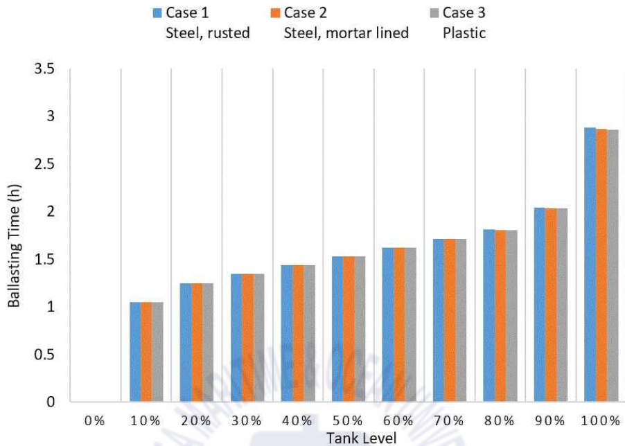
Fig. 3-4 Ballasting time calculation as per the different pipe materials for 325K VLOC
